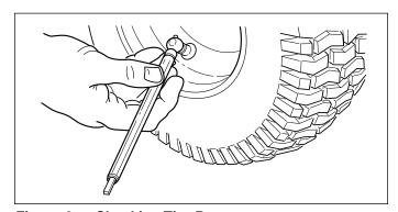
Figure 2. Checking Tire Pressure
